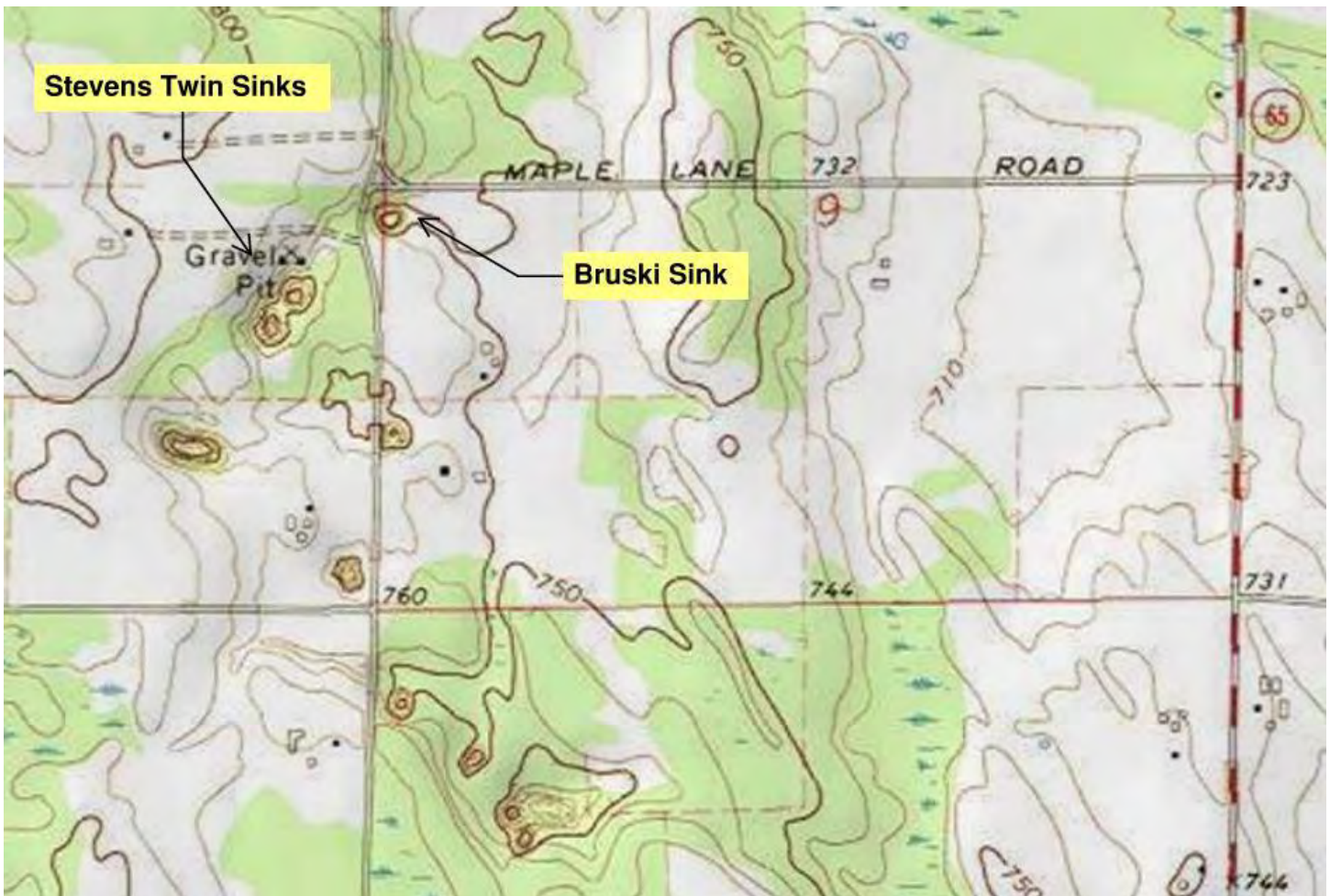
Figure 2: USGS topographic map of Bruski and Stevens Twin Sinks. Note the additional sinkholes in the surrounding area, and the near perpendicular orientation of the sinkhole groups, suggesting development of the sinkholes along joint patterns in the bedrock.
