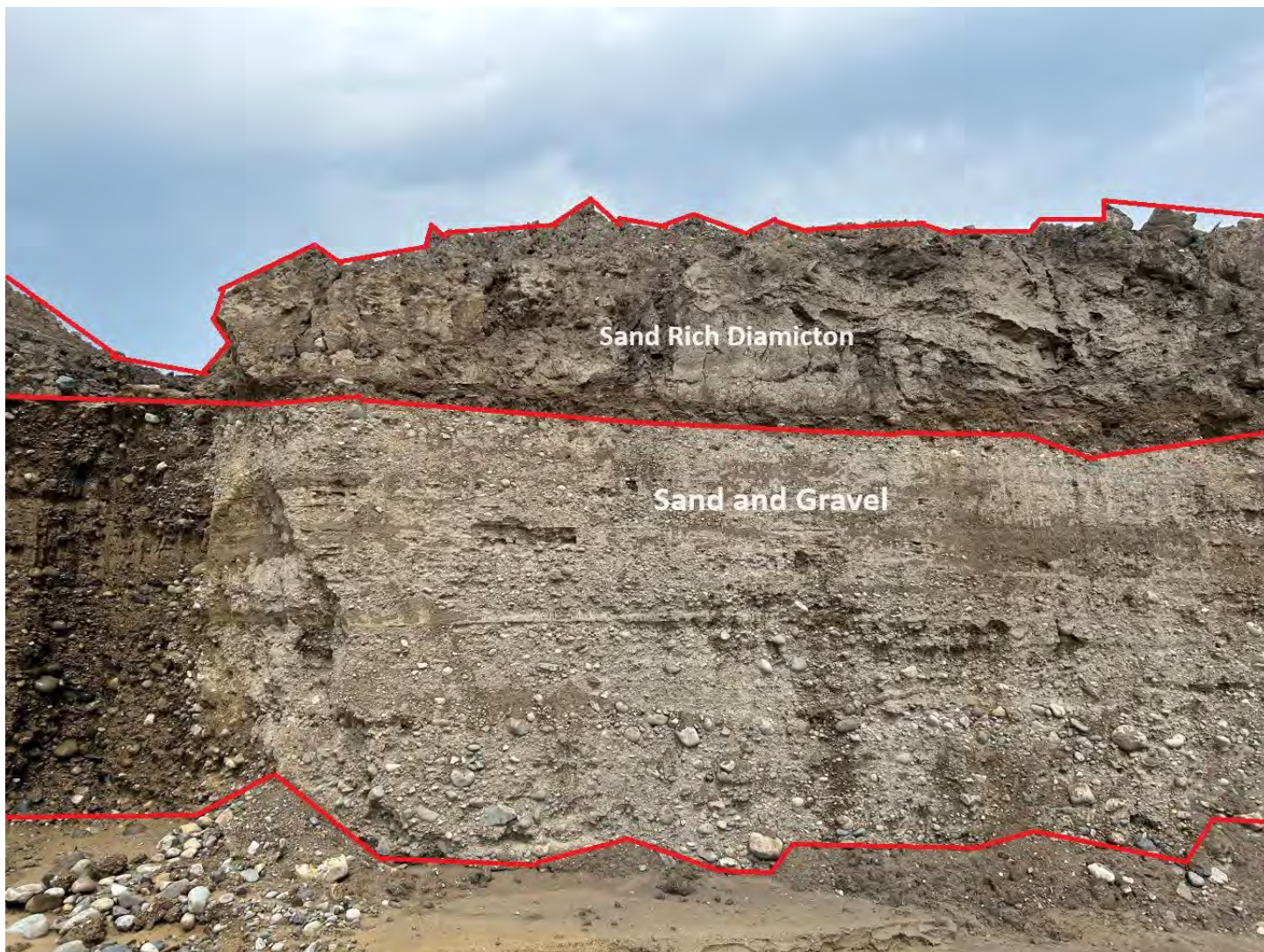
Image 1: This photo was taken facing west. Glacial outwash exposure at Koenig Materials located at 1955 East Lakeville, MI. The upper unit is an approximately ten feet thick, gray and brown sand-rich diamiction. Beneath this unit is brown sand, fine to coarse grained, gravel is small to large and rich in igneous and metamorphic cobbles and boulders. This unit is well to poorly sorted, well stratified, in places cross-bedded sand lens. This unit is approximately 15 feet thick. The entire outcrop is approximately 25 feet. Photo taken by Ira Adolphues .
