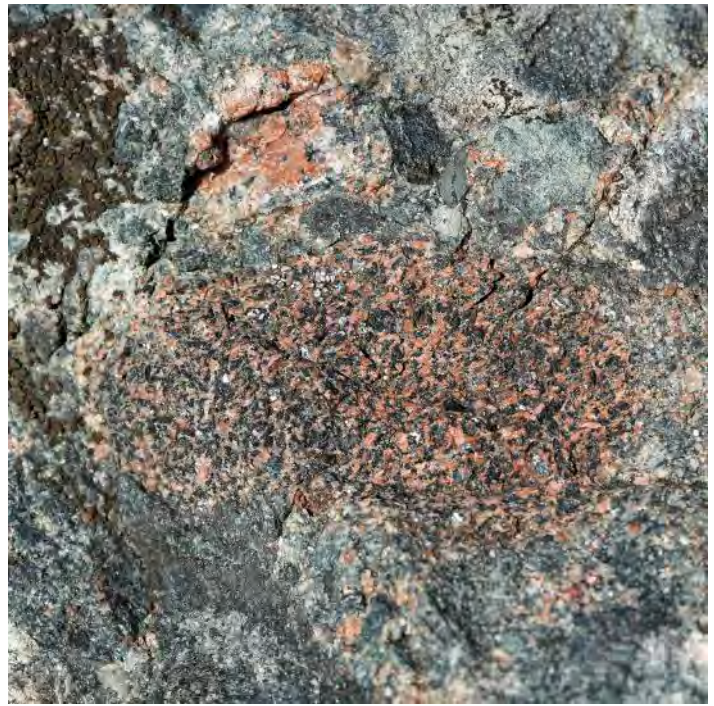
Figure 12: An elongated fine-grained red granite with muscovite mica and hornblende crystals. Approximately three inches in length.
