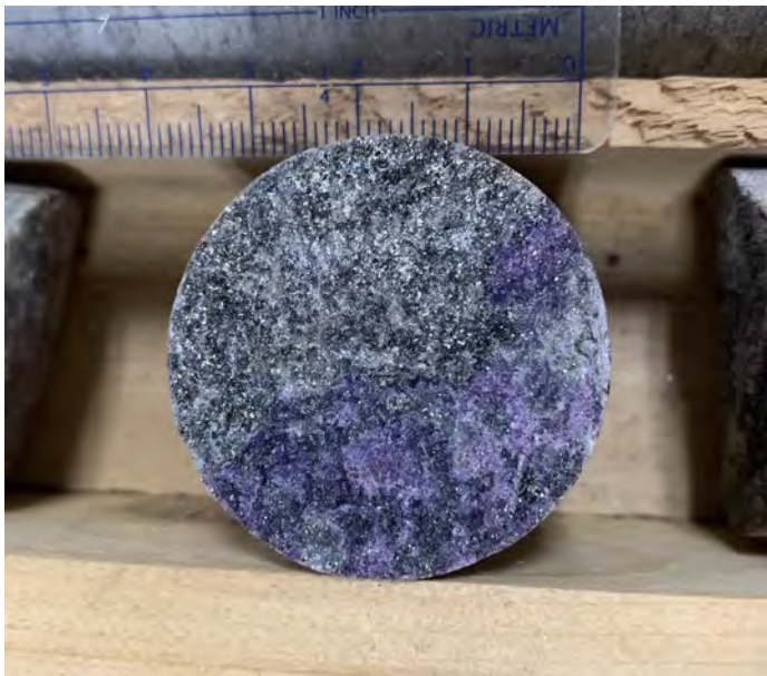
Figure 5: Drill core with anomalous fluorite (purple) mineralization in gneiss from the Watersmeet gneiss dome, Gogebic county.
