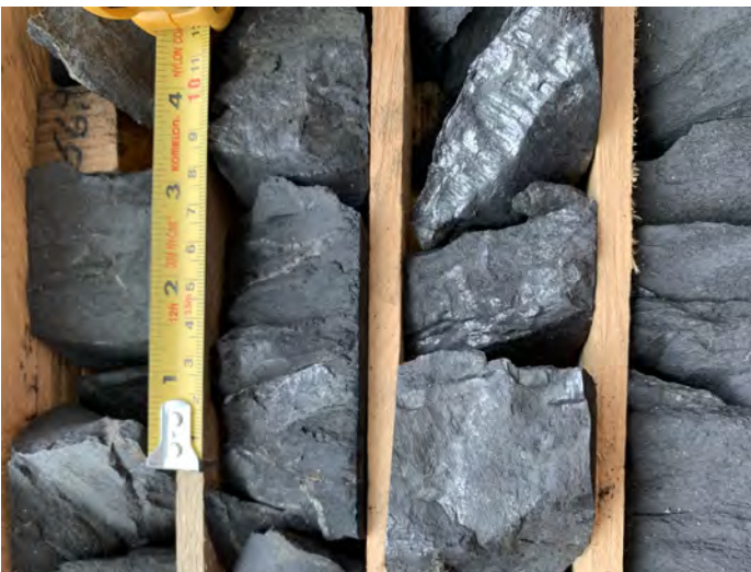
Figure 3: Graphite-bearing drill core from the Lower Slate Member.
