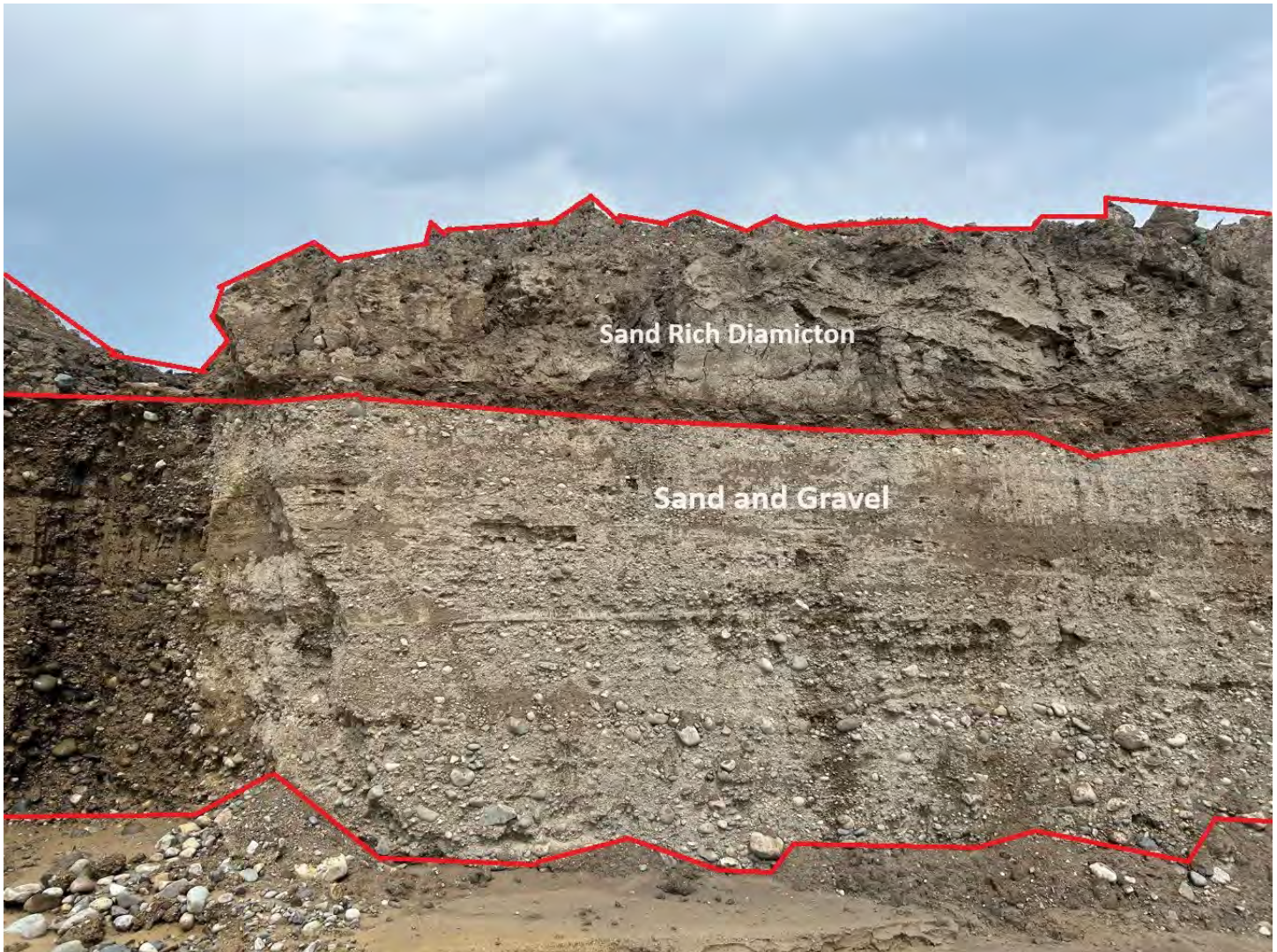
Image 1: This photo was taken facing west. Glacial outwash exposure at Koenig Materials located at 1955 East Lakeville, MI. The upper unit is an approximately ten feet thick, gray and brown sand-rich diamicton. Beneath this unit is brown sand, fine to coarse grained, gravel is small to large and rich in igneous and metamorphic cobbles and boulders. This unit is well to poorly sorted, well stratified, in places cross-bedded sand lens. This unit is approximately 15 feet thick. The entire outcrop is approximately 25 feet. Photo taken by Ira Adolphues .
