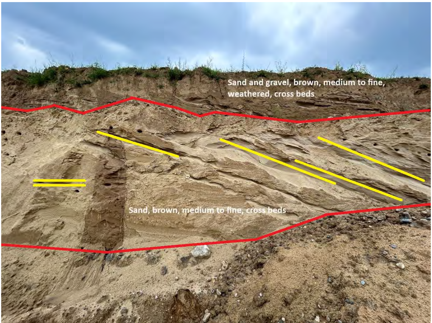
Image 2: This photo was taken facing south. The upper unit is sand and gravel, brown, medium to fine grained, with cross beds. This upper unit exhibits some weathering. The lower unit is sand, brown, fine to medium grained, and contains cross beds. Photo by taken Ira Adolphues .
