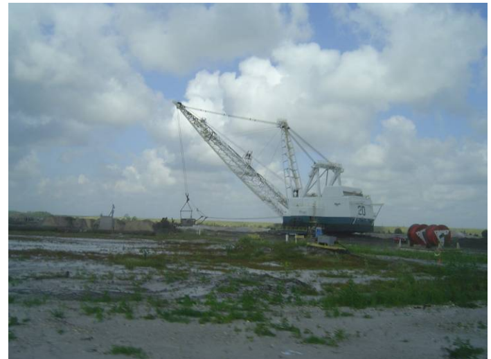
The phosphate mining drag line with its 55 cubic yard "bucket" in action. Photograph courtesy of Adam Heft.
